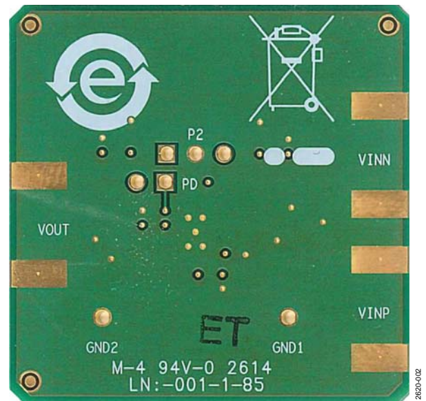
Figure 2. SO8 SINGLE AMP Evaluation Board, Secondary Side
