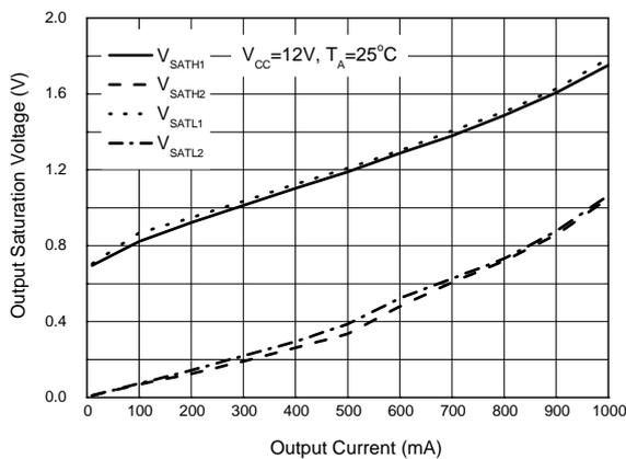
Figure 6. Output Saturation Voltage vs. Output Current
