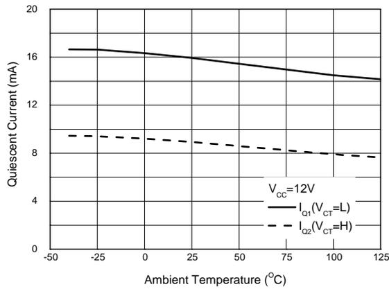
Figure 4. Quiescent Current vs. Ambient Temperature
