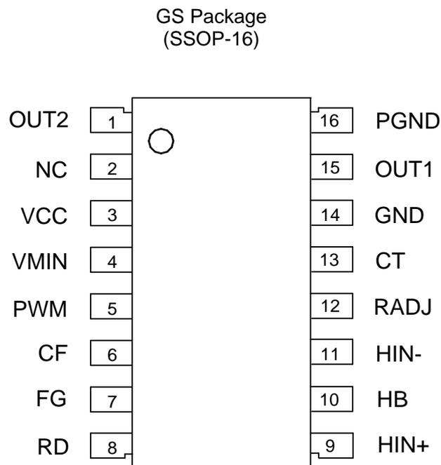
Figure 2. Pin Configuration of AM4962 (Top View)
