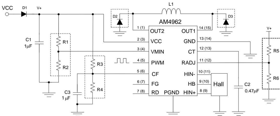
**Application 2 (Slope K and Minimum/Maximum Duty Adjustable)**
