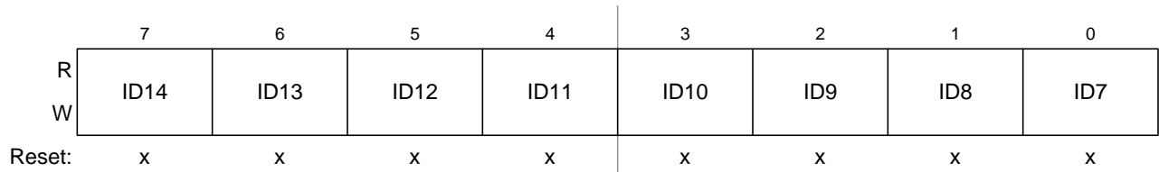
Figure 12-28. Identifier Register 2 (IDR2) — Extended Identifier Mapping
