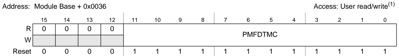
Figure 14-38. PMF Deadtime C Register (PMFDTMC)
