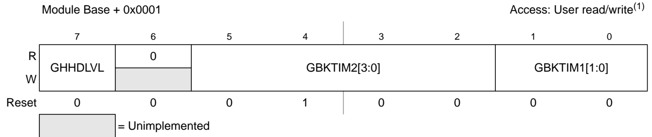
Figure 17-4. GDU Control Register (GDUCTR)
