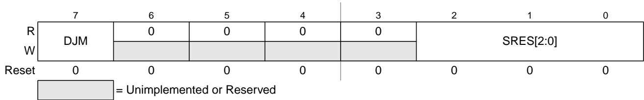
Figure 9-8. ADC Format Register (ADCFMT)
