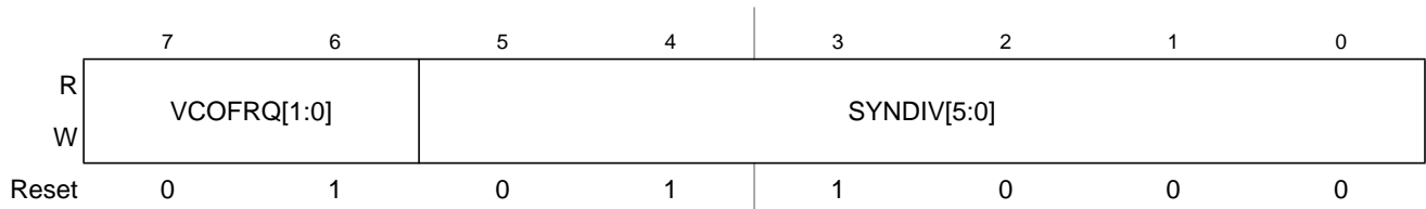
Figure 8-5. S12CPMU_UHV_V6 Synthesizer Register (CPMUSYNR)
