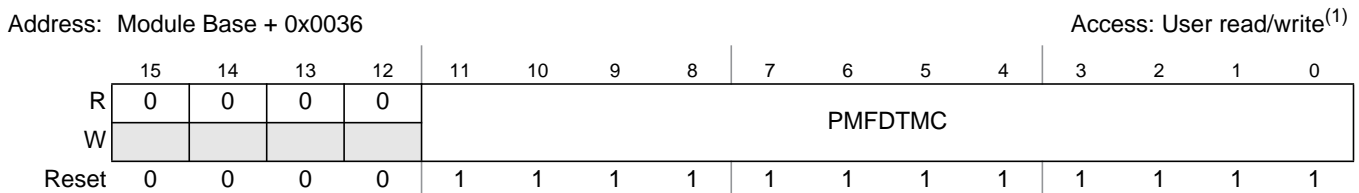
Figure 14-38. PMF Deadtime C Register (PMFDTMC)
