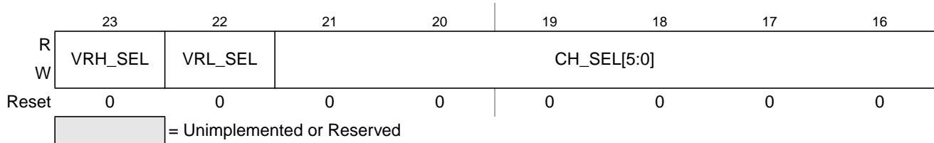
Figure 9-19. ADC Command Register 1 (ADCCMD_1)
