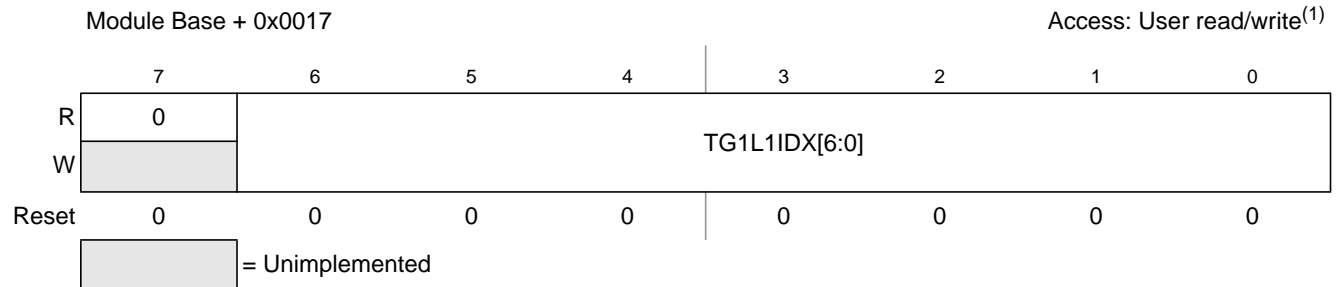
Figure 13-20. Trigger Generator 1 List 1 Index (TG1L1IDX)
