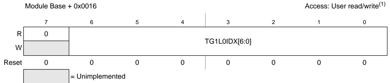
Figure 13-19. Trigger Generator 1 List 0 Index (TG1L0IDX)
