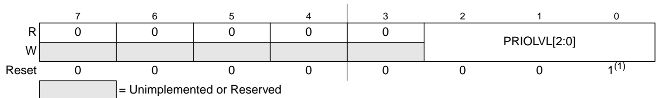
Figure 4-8. Interrupt Request Configuration Data Register 3 (INT_CFDATA3)
