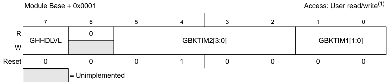
Figure 17-4. GDU Control Register (GDUCTR)
