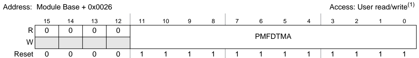
Figure 14-28. PMF Deadtime A Register (PMFDTMA)
