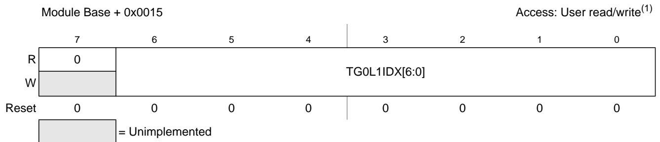
Figure 13-18. Trigger Generator 0 List 1 Index (TG0L1IDX)
