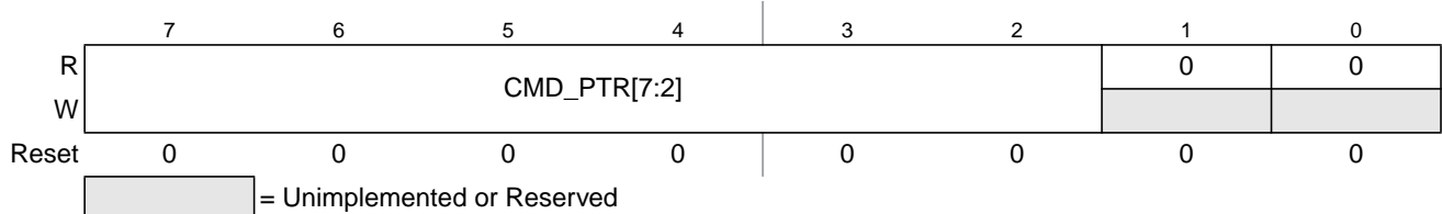
Figure 9-23. ADC Command Base Pointer Registers (ADCCBP_0, ADCCBP_1, ADCCBP_2)
