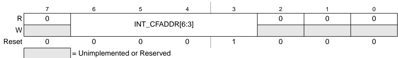
Figure 4-4. Interrupt Configuration Address Register (INT_CFADDR)
