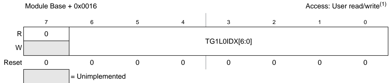
Figure 13-19. Trigger Generator 1 List 0 Index (TG1L0IDX)
