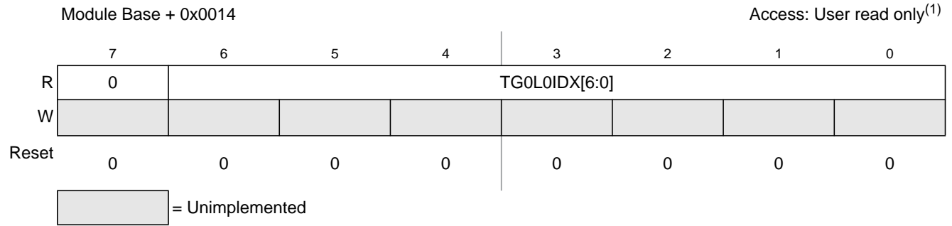
Figure 13-17. Trigger Generator 0 List 0 Index (TG0L0IDX)
