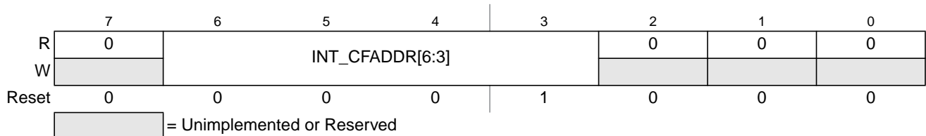
Figure 4-4. Interrupt Configuration Address Register (INT_CFADDR)
