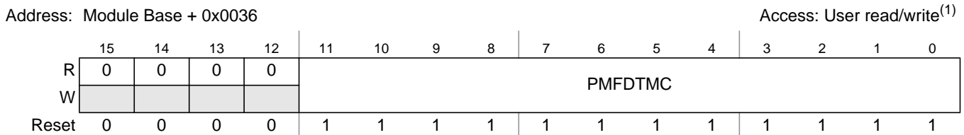
Figure 14-38. PMF Deadtime C Register (PMFDTMC)
