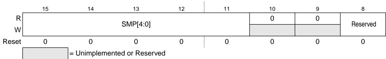
Figure 9-20. ADC Command Register 2 (ADCCMD_2)
