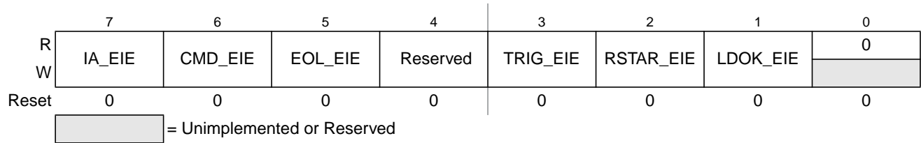
Figure 9-10. ADC Error Interrupt Enable Register (ADCEIE)
