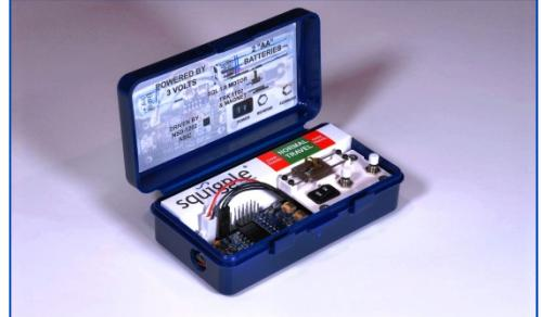
Developer's kits demonstrate system performance of an integrated SQUIGGLE motor, NSD-2101 driver and NSE-5310 position sensor.
