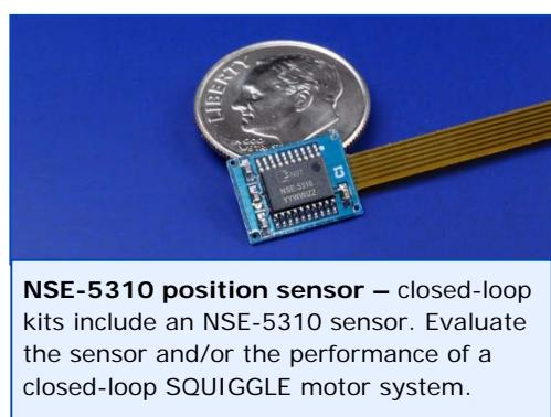
**NSE-5310 position sensor** – closed-loop kits include an NSE-5310 sensor. Evaluate the sensor and/or the performance of a closed-loop SQUIGGLE motor system.
