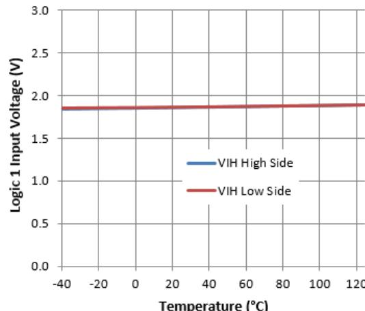
Figure 22. Logic 1 Input Voltage vs. Temperature
