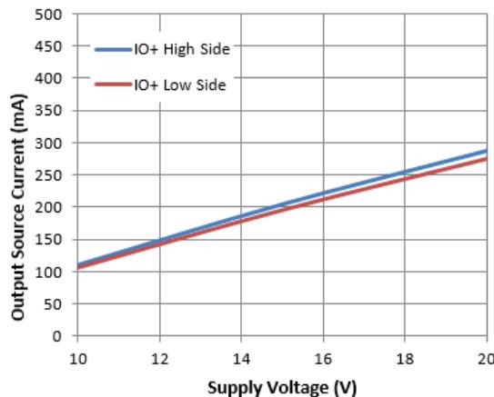
Figure 17. Output Source Current vs. Supply Voltage
