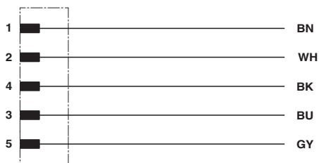
Contact assignment of the M12 plug
