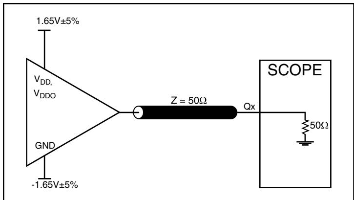
3.3V Core/3.3V LVCMS Output Load AC Test Circuit
