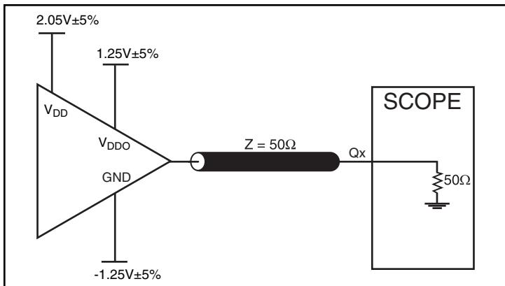
3.3V Core/2.5V LVCMS Output Load AC Test Circuit
