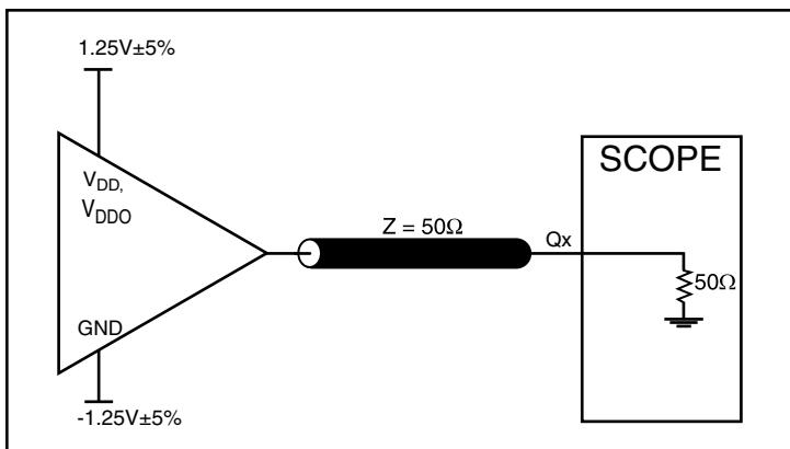
2.5V Core/2.5V LVCMS Output Load AC Test Circuit
