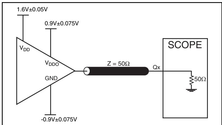
2.5V Core/1.8V LVCMS Output Load AC Test Circuit
