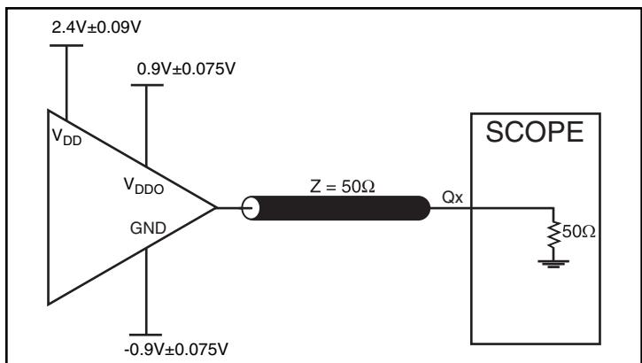
3.3V Core/1.8V LVCMS Output Load AC Test Circuit
