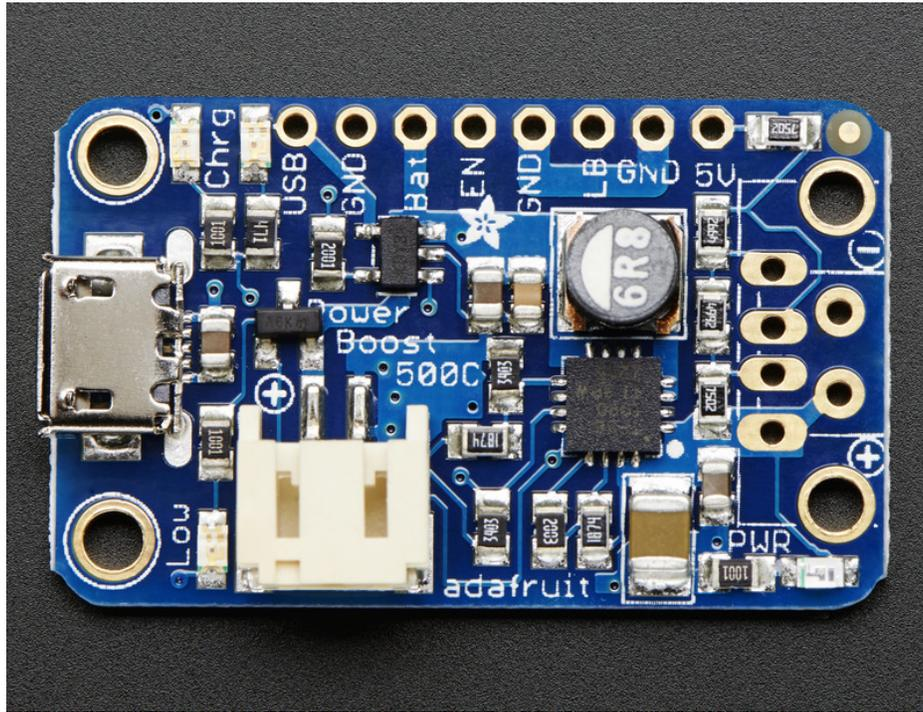
The PowerBoost 500C has at the heart a [TPS61090 boost converter from TI](https://adafru.it/duQ) (<https://adafru.it/duQ>). This boost converter chip has some really nice extras such as low battery detection, 2A internal switch, synchronous conversion, excellent efficiency, and 700KHz high-frequency operation. Check out these specs!
