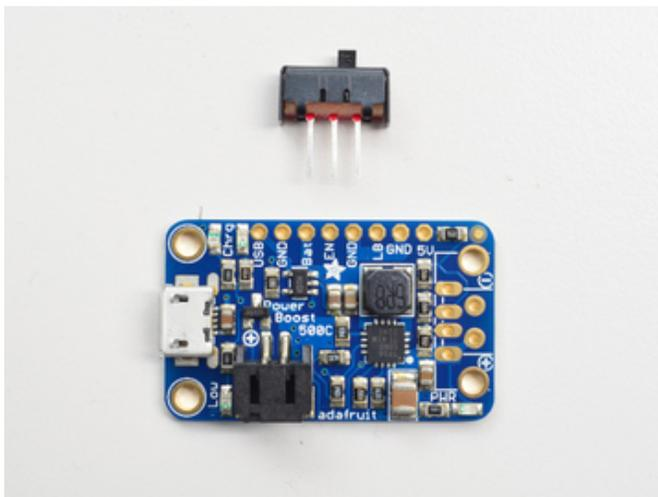
The switch will go into the breakout header, and attach to **VBAT EN** and **GND**
