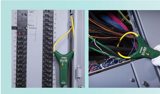
Flexible clamp jaw easily wraps around bus bars and cable bundles that may be difficult to access with regular clamp meters. The thin 7.5mm cable diameter easily fits into tight spaces. Choose between a 10" (25.4cm) or 18" (45.7cm) cable clamp length to accommodate your application needs.
