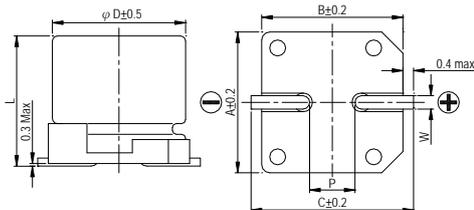
Lead Spacing and Diameter Unit: mm
