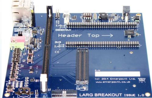
The Larg Breakout Board supports your development process and it also allows FMC modules to be used in conjunction with Larg2. This low cost design demonstrates the cost effectiveness of Larg2 in real applications.
