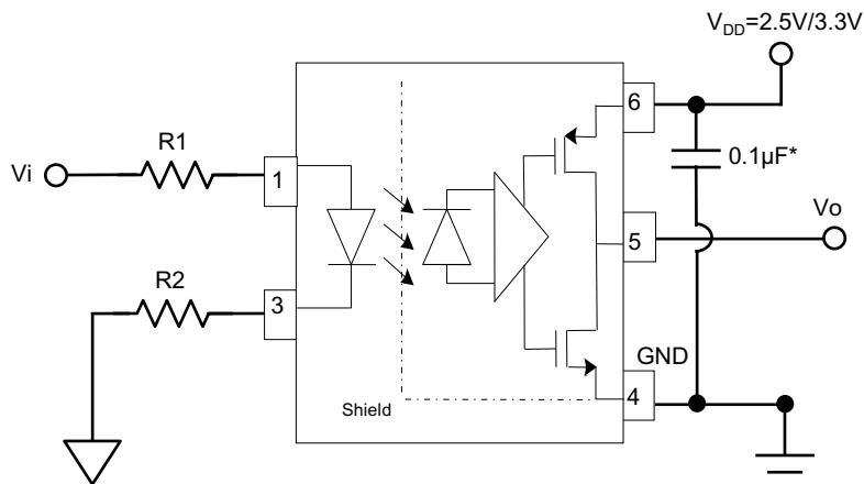
\* Bypass capacitor at no more than 3 mm from optocoupler's power pins ( $V_{DD}$ , GND).
