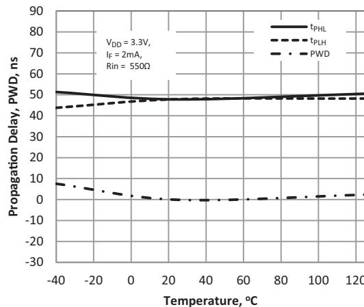
**Figure 11: Typical Switching Timing (Propagation Delay, PWD) vs Temperature at 3.2-mA LED Driving Current, 3.3V Supply**
