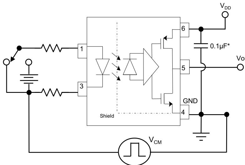
\* Bypass capacitor at no more than 3 mm from optocoupler's power pins ( $V_{DD}$ , GND).
