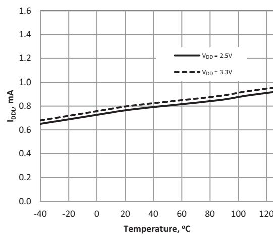
**Figure 5: Typical Logic High Output Supply Current  $I_{DDH}$  vs. Temperature**
