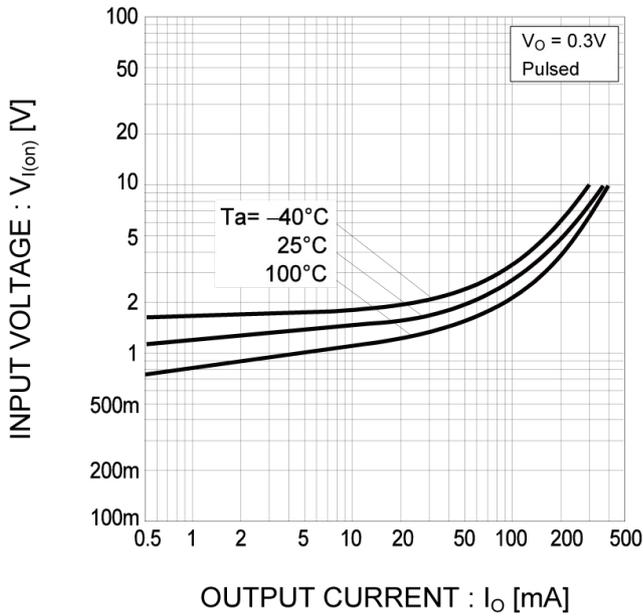
Fig.2 Output Current vs. Input Voltage (OFF Characteristics)
