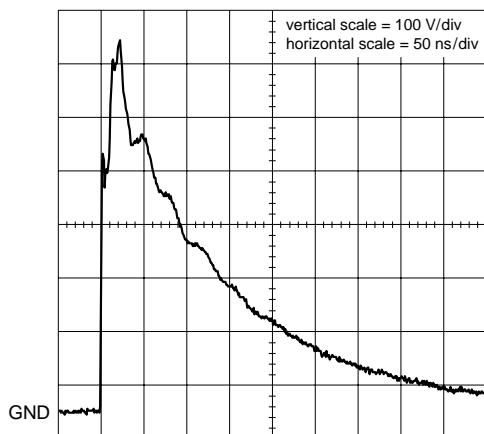
unclamped +1 kV ESD voltage waveform
