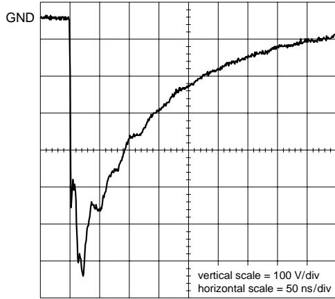
unclamped -1 kV ESD voltage waveform
