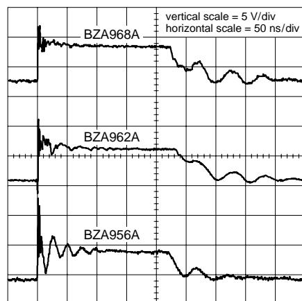
clamped +1 kV ESD voltage waveform
