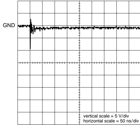
clamped -1 kV ESD voltage waveform
