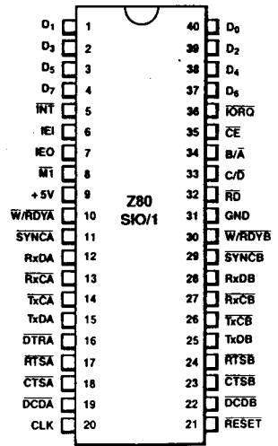
Figure 4. 40-pin Dual-In-Line Package (DIP), Pin Assignments
