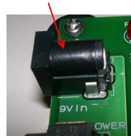
(3) Soldering the DC Power Jack
