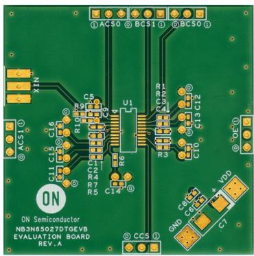
**Figure 3. Evaluation Board top View (Bare PCB)**
