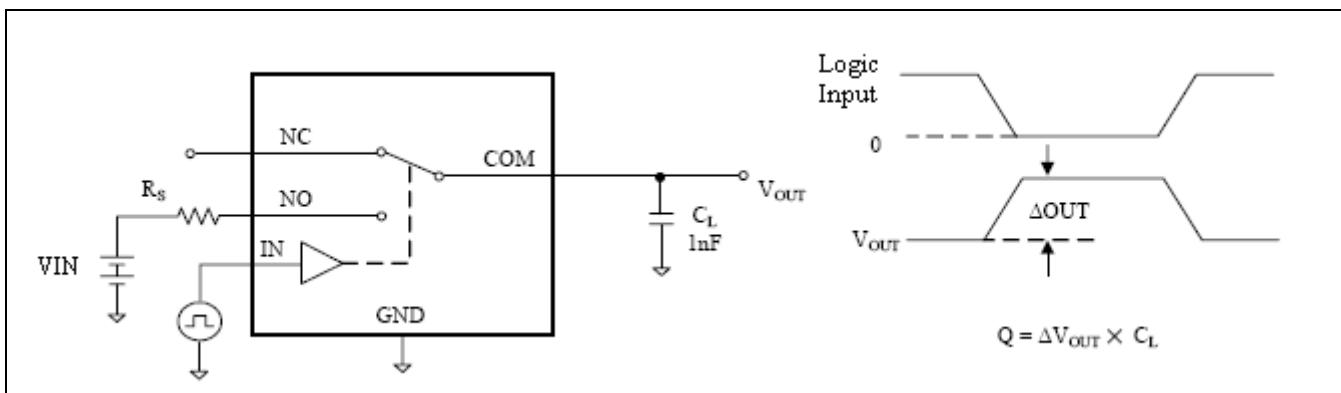
**Figure 8. Charge Injection**
