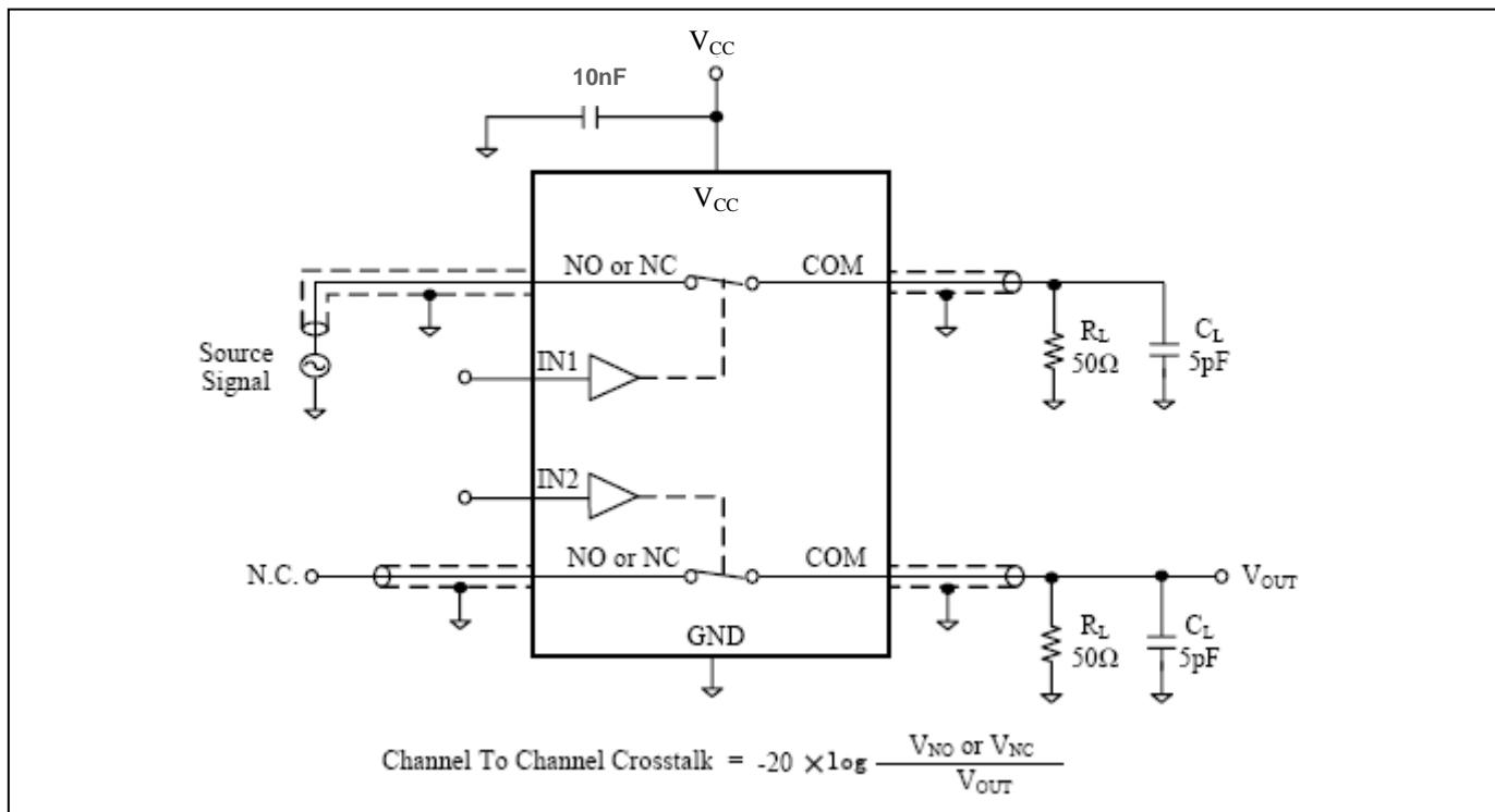
**Figure 6. Channel-to-Channel Crosstalk**
