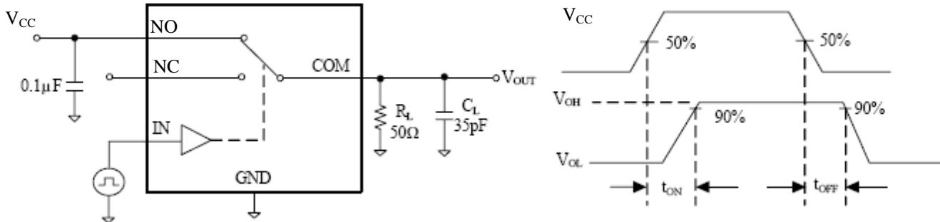
Figure 2. Switching Times
