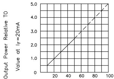
Relative Radiant Intensity Vs. Forward Current
