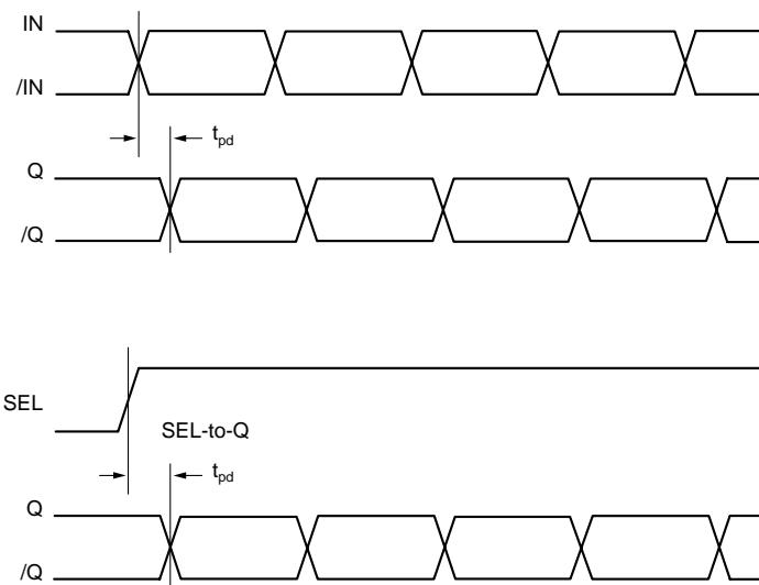
Figure 2. Timing Diagram
