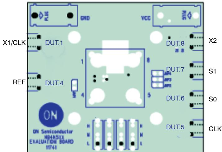
Figure 7. NB3N502 Evaluation Board SMA – Ground Layer
