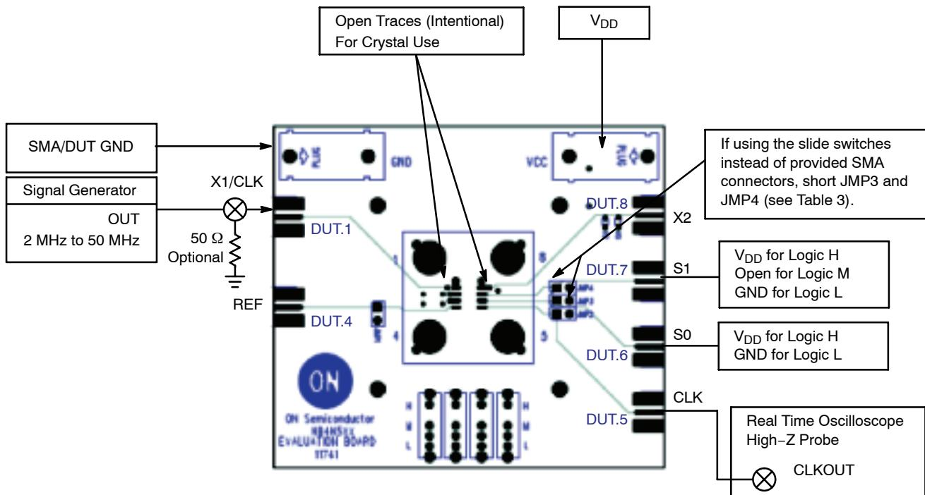
**Figure 5. Typical Setup**
