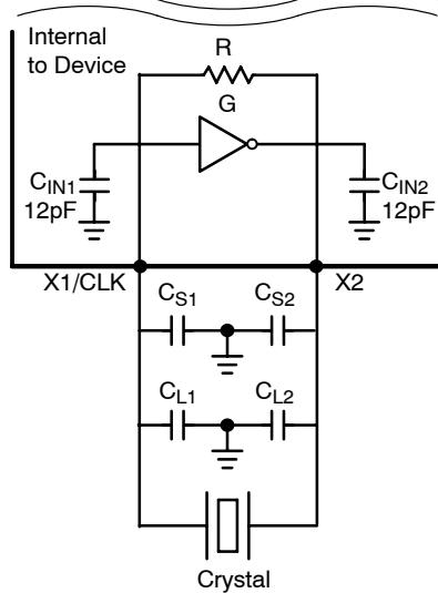
**Figure 3. Using a Crystal as Reference Clock**
