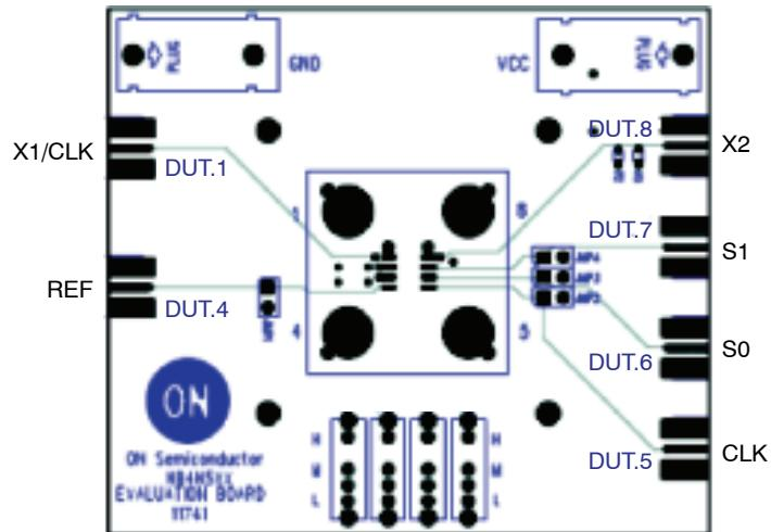
Figure 6. NB3N502 Evaluation Board Top (Component) Layer
