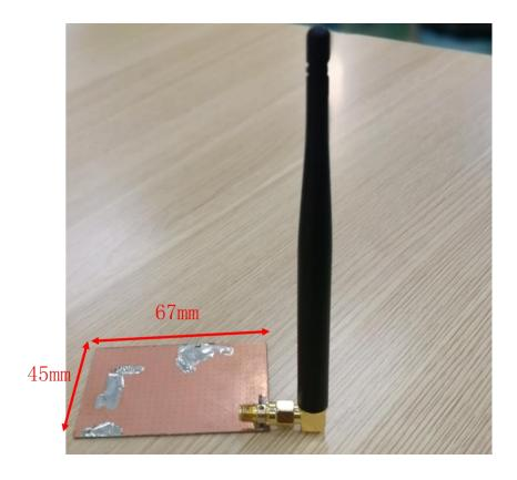
Test with a 45mm\*67mm ground plane in free space.
