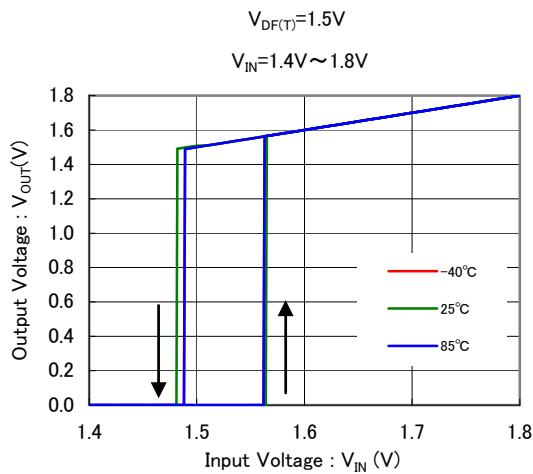
(4) Detect Voltage, Release Voltage
