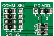
Pressure 2 click™ carries two sets of jumpers [zero ohm resistors]. The group of four COMM. SEL jumpers is for choosing between SPI or I2C interface. I2C ADD is for specifying the I2C address.
