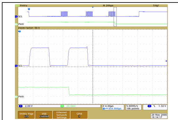
FIGURE 2-63: 50\text{ k}\Omega – Low-Voltage Decrement Wiper Settling Time ( V_{DD} = 5.5\text{V} ) ( 1\text{ }\mu\text{s/Div} ).
