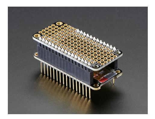
But don't forget, you can also put the stacking headers on the Proto wing and stack the Feather on top of it!
