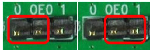
The output enable pins can be changed on the fly to observe outputs stopped cleanly. To enable the spread spectrum, the SSON input needs to change from a logic level low to high. Input functionality is explained in detail below.
