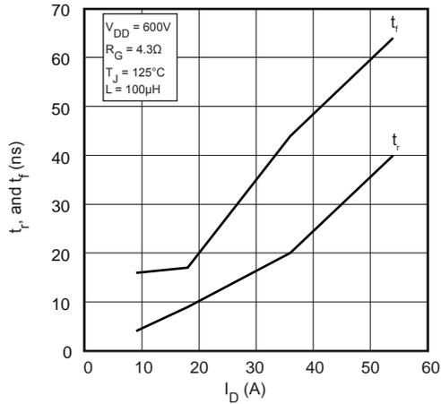
FIGURE 14, Rise and Fall Times vs Current
