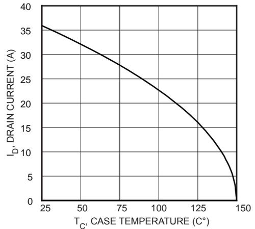
FIGURE 5, Maximum Drain Current vs Case Temperature
