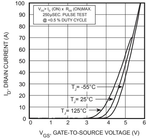
FIGURE 3, Transfer Characteristics
