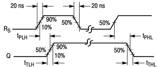
**Figure 2. Switching Time Test Circuit and Waveforms**
