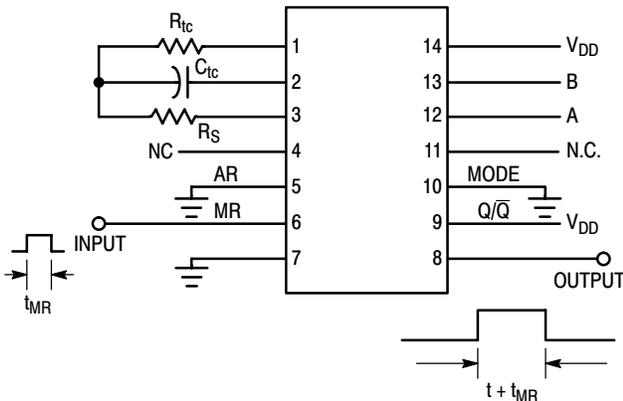
When Master Reset (MR) receives a positive pulse, the internal counters and latch are reset. The Q output goes high and remains high until the selected (via A and B) number of clock pulses are counted, the Q output then goes low and remains low until another input pulse is received.
