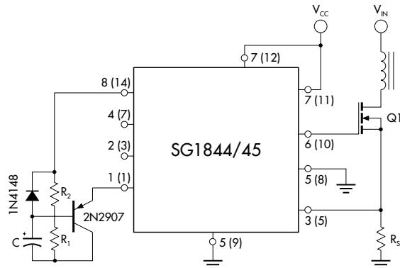
$$I_{PK} = \frac{V_1}{R_S} \quad \text{Where: } 0 \leq V_1 \leq 1.0V \quad t_{SOFTSTART} = -\ln 1 \left[ -\frac{V_C}{V_2} \right] C \frac{R_1 R_2}{R_1 + R_2}$$
