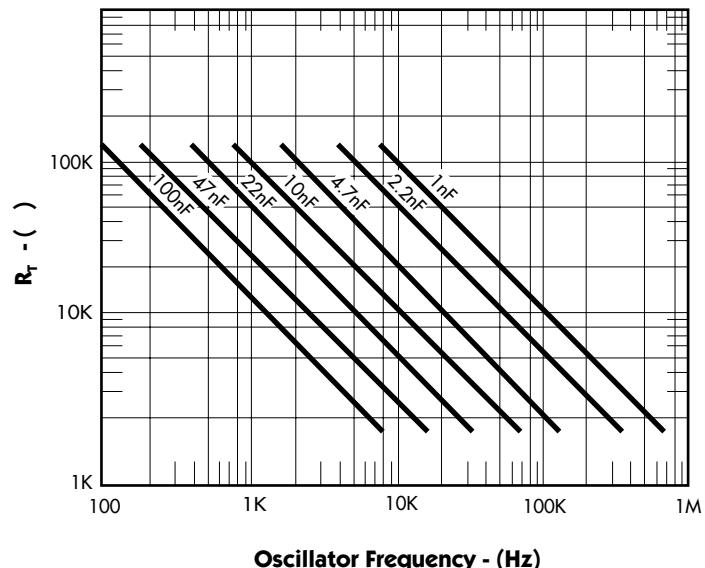
FIGURE 13 — OSCILLATOR FREQUENCY vs.  $R_T$  FOR VARIOUS  $C_T$
