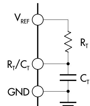
$$F \approx \frac{1.86}{R_T C_T} \text{ where } R_T \geq 5\text{k}\Omega$$
