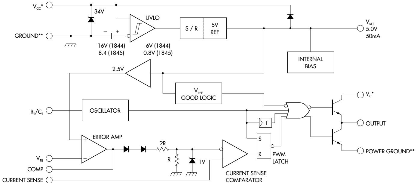
\* -  $V_{CC}$  and  $V_c$  are internally connected for 8-pin packages.
