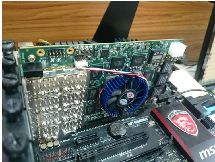
Figure 7-9 FPGA board installation on PC
