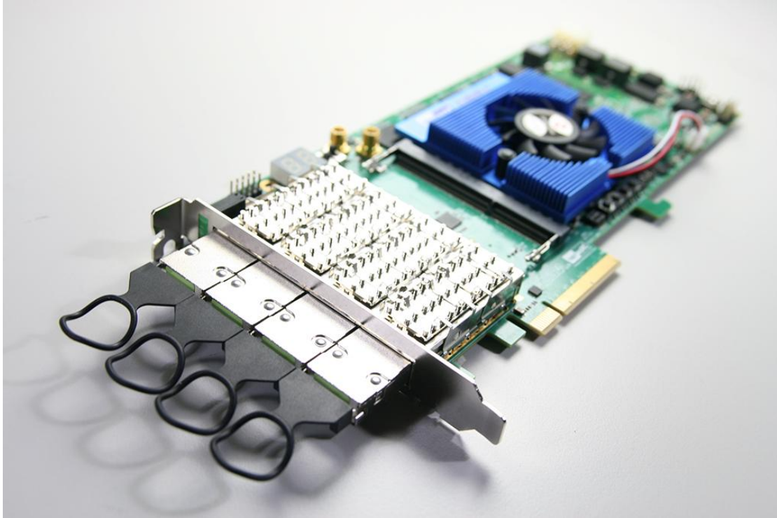
Figure 8-4 Four QSFP+ Loopback Fixtures Installed
