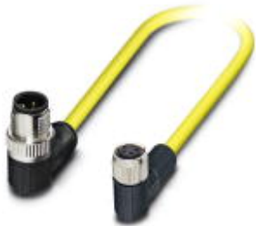
Sensor/Actuator cable, 4-position, PVC, Yellow RAL 1021, Plug angled M12-SPEEDCON, A-coded, on Socket angled M8, Cable length: 1.5 m
