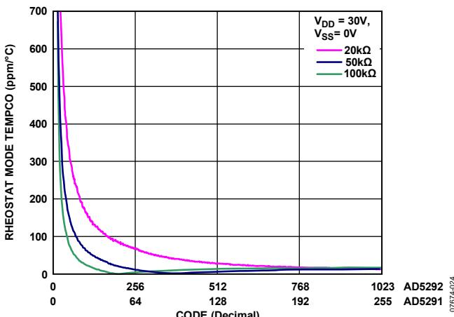
Figure 38. Rheostat Mode Tempco  $\Delta R_{WB}/\Delta T$  vs. Code
