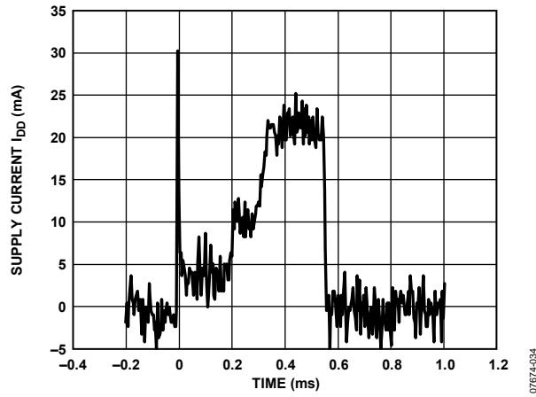
Figure 49.  $I_{DD}$  Waveform While Blowing/Reading Fuse
