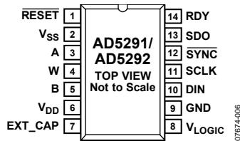
Figure 5. Pin Configuration
