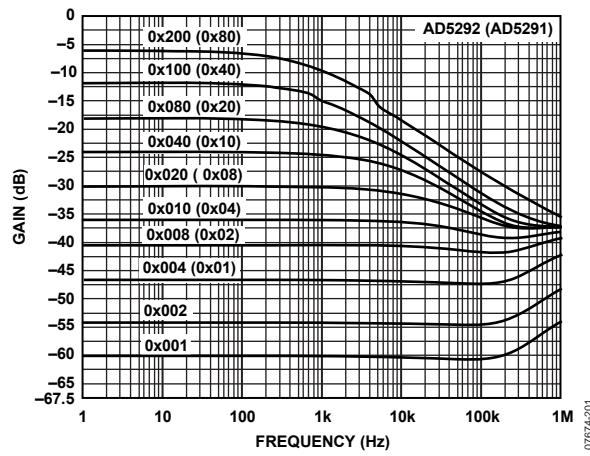
Figure 45. 100 k $\Omega$  Gain vs. Frequency vs. Code
