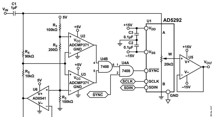
Figure 74. Audio Volume Control with Zipper Noise Reduction
