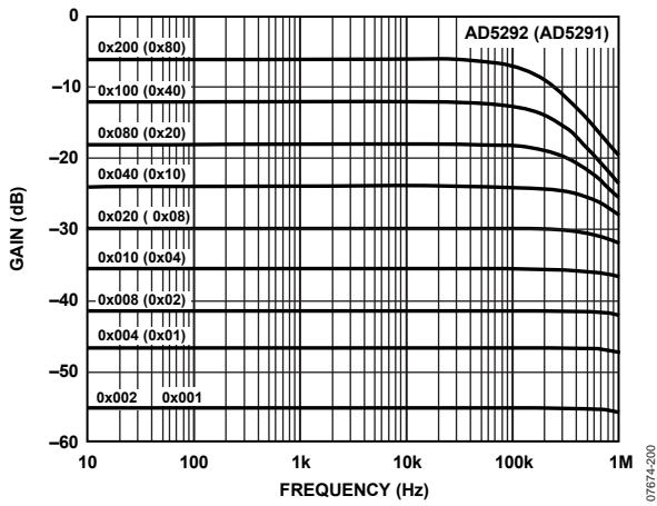
Figure 43. 50 k $\Omega$  Gain vs. Frequency vs. Code
