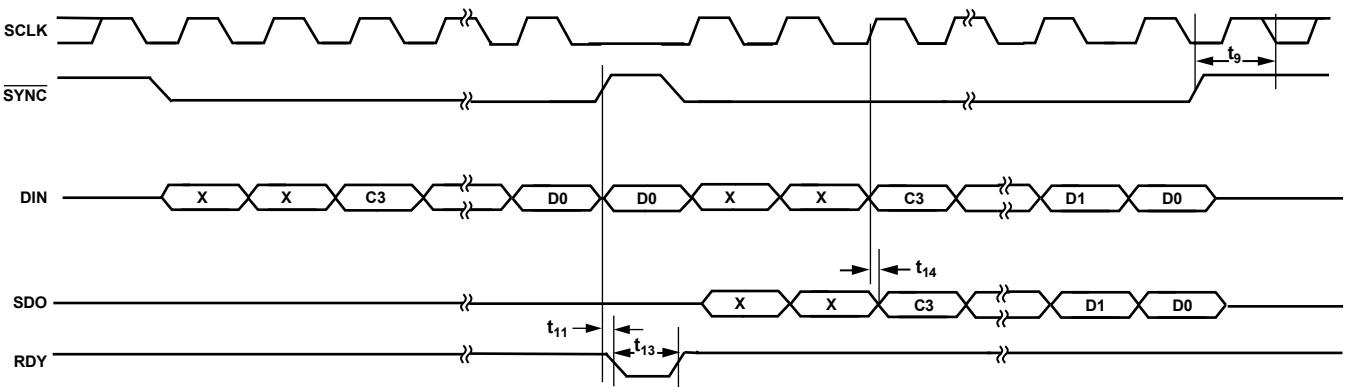
Figure 4. Read Timing Diagram, CPOL = 0, CPHA = 1
