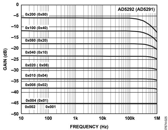
Figure 42. 20 k $\Omega$  Gain vs. Frequency vs. Code
