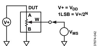
Figure 59. Potentiometer Divider Nonlinearity Error
