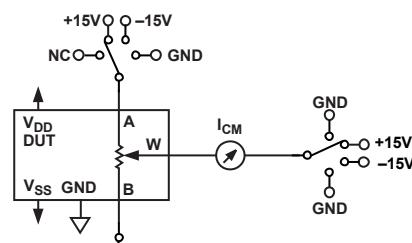
Figure 63. Common-Mode Leakage Current
