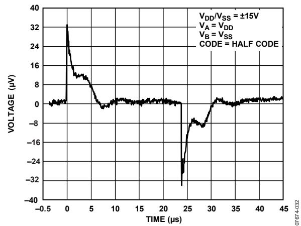
Figure 53. Digital Feedthrough
