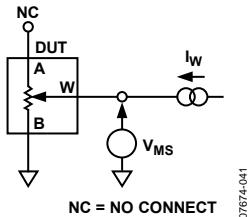
Figure 58. Resistor Position Nonlinearity Error
