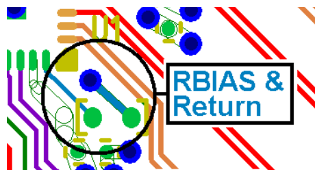
Figure 3.7 RBIAS Return Routing
