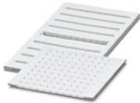
Flat zack marker sheet, Sheet, white, Labeled, Printed horizontally: Consecutive numbers from 1 - 100, Mounting type: Snap into flat marker groove, For terminal block width: 4.2 mm, Lettering field: 4.2 x 5.2 mm
