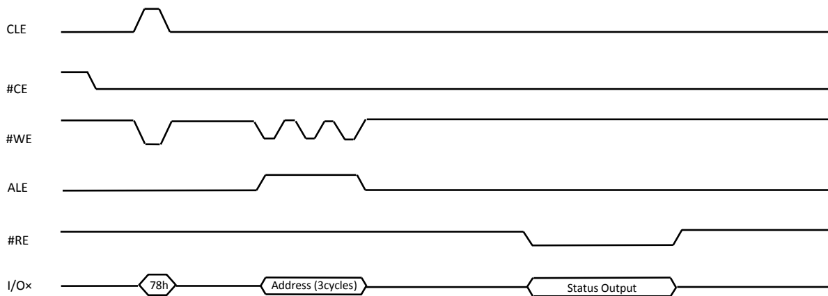
Figure 9-10 Read Status Enhanced (78h) Operation
