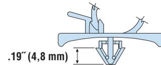
Release tab provides easy opening without forcing.
