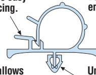
Quick lock/release allows fast lock-up and easy access to wire bundle.
