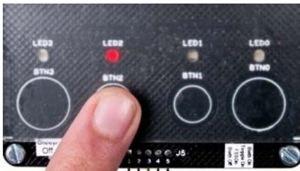
1. Touch a button; LED turns on
