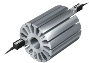
Thickness measurement of motor cores
