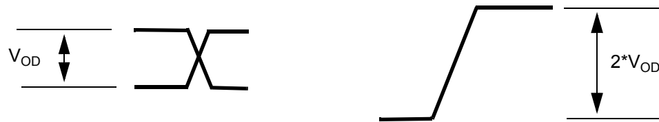
Figure 19 - Differential Voltage Parameter
