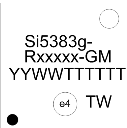
Figure 12.1. Si5383 Top Marking
