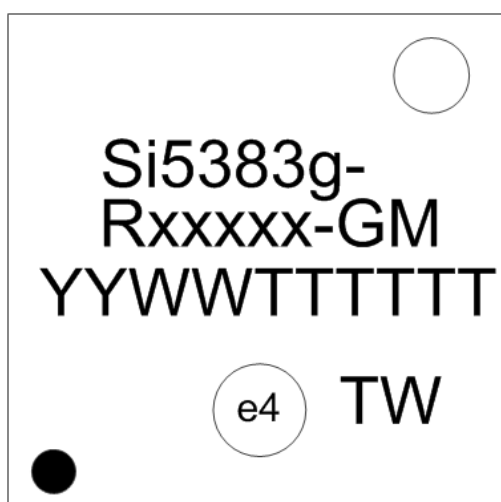
Figure 12.1. Si5383 Top Marking
