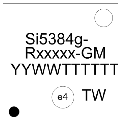
Figure 12.2. Si5384 Top Marking
