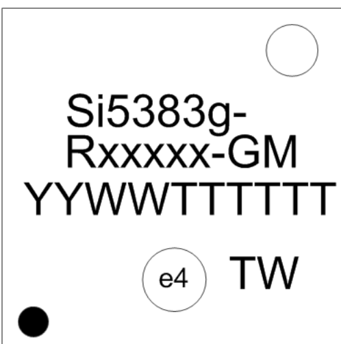
Figure 12.1. Si5383 Top Marking
